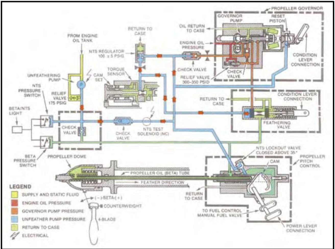
Figure 1 – NTS Start Check Powered by Unfeather Pump
